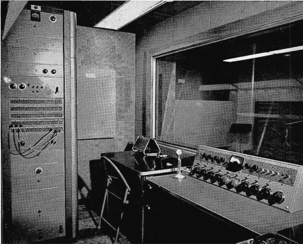
FIG. 7. Studio C's Console has many desirable features for a functional program studio. This RCA Custom-Built Console is equipped to handle four microphone inputs, two turntables, and facilities for remotes 1-2, 3-4, and a network control. A special feature is the Echo Effects circuit built into the console, highly desirable for dramatic programs.
