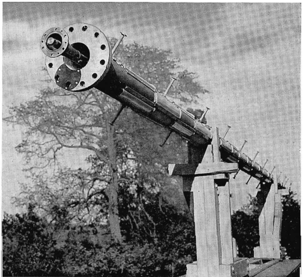
FIG. 3. Bottom View of TFU-24-BH Antenna Mounted on Turntable for Vertical Pattern Measurements, Showing Mounting Flange and Transmission Line Connection.
