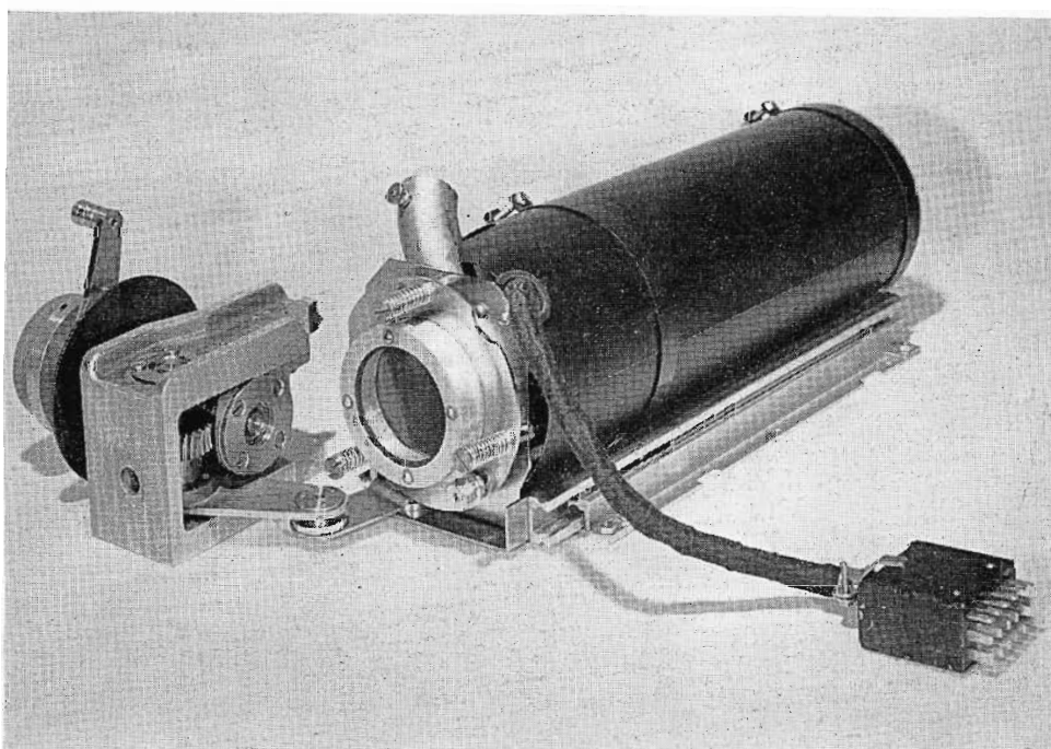
FIG. 8. Yoke assembly and focus drive mechanism removed from the camera. Note blower hose fitting and plug for electrical connections.
